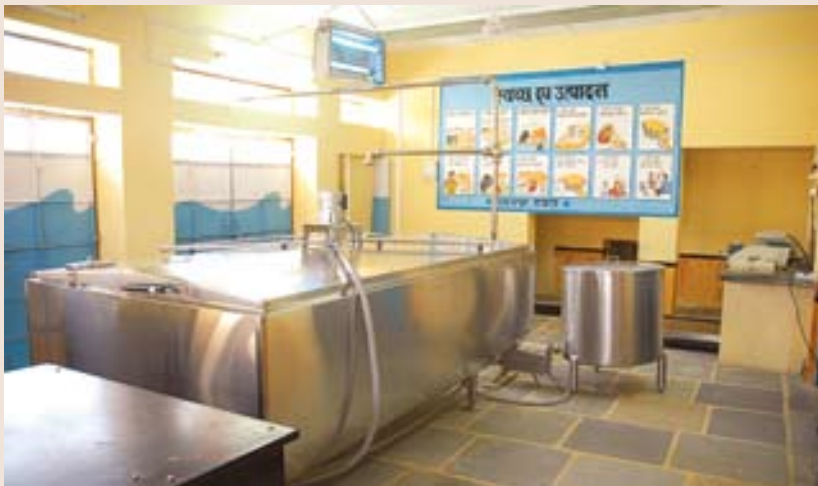
A Bulk Milk Cooler of 5000 Litre Capacity Installed at a Dairy Cooperative Society in Rajasthan
